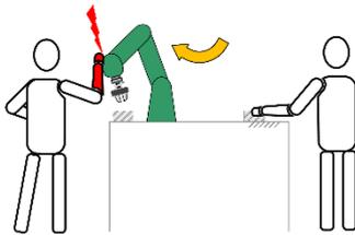
“fence-less” applications: access to moving devices (and potential hazards) is not prevented by perimeter safeguarding, BUT risks are mitigated by collaborative features:
