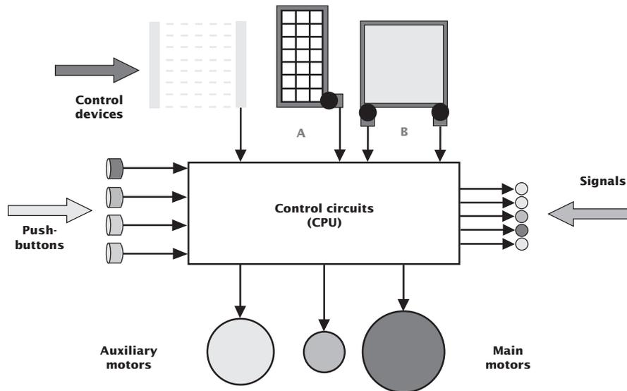
Even the simplest machine's control system carries out different functions, each controlled by a specific combination of hardware and software elements.
