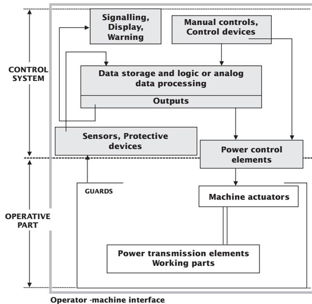
While this distinction is correct in principle, it should be borne in mind that the designer allocates safety functions to the control system as a combination of communicating hardware and software, with separate and/or integrated components.
