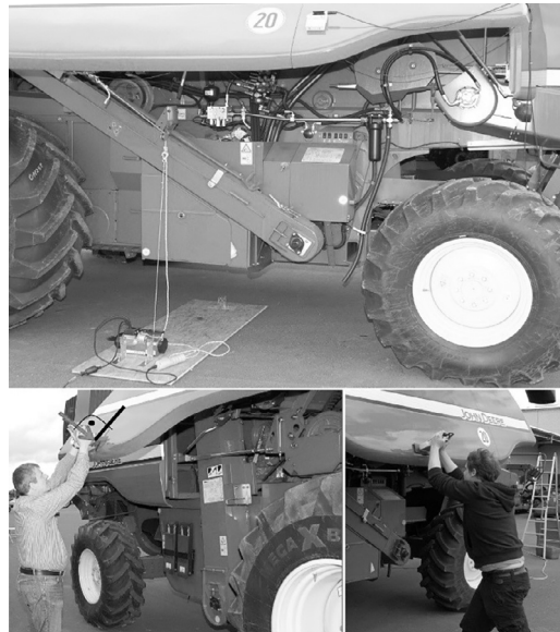
Figure 2 Automatic (top) and manual measuring procedure with two examiners (bottom)
